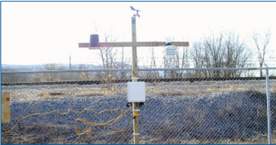
Weather station installed to support an ambient air monitoring program. Wind speed and direction data were among the measured parameters.
