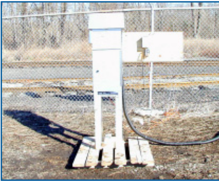
High-volume sampler used for collection of ambient air samples for analysis of PAHs.
